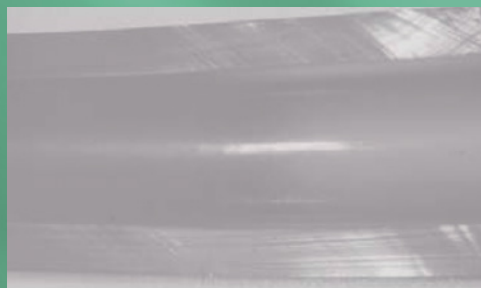
Silclear tubing after over 54 months use
